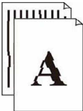
Lines Are Misaligned/Distorted
